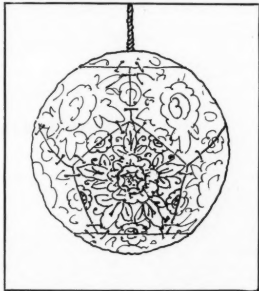
TWELVE SECTIONS OF FIVE SIDED MOULDED SATIN FINISHED GLASS, WIRED TOGETHER MADE A BEAUTIFUL LUMINOUS BALL. A VERY INGENUOUS CONSTRUCTION GIVING AN EXCELLENT RESULT AT A MINIMUM COST FOR MODELS
